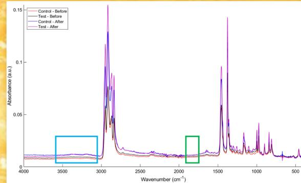
FTIR spectra of aged and unaged samples of unpigmented PP showing no changes after ageing in the hydroxyl (blue box) or carbonyl (green box) regions which would indicate photooxidation of the polymer.
