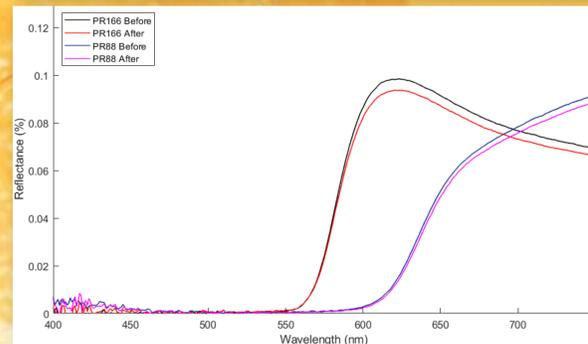
Visible reflectance spectra of the two red PP samples showing no shifts in the reflectance curves which would indicate colour change of the materials after ageing.
