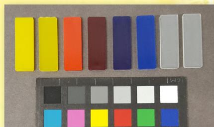
PP samples used in the first experiment. From left to right: PY95, PY83, PR166, PR88, PB15:1, PB29, unpigmented PP.
